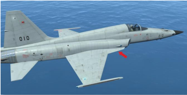
Wing leading edge extension. (Flaps fully retracted - UP position)
