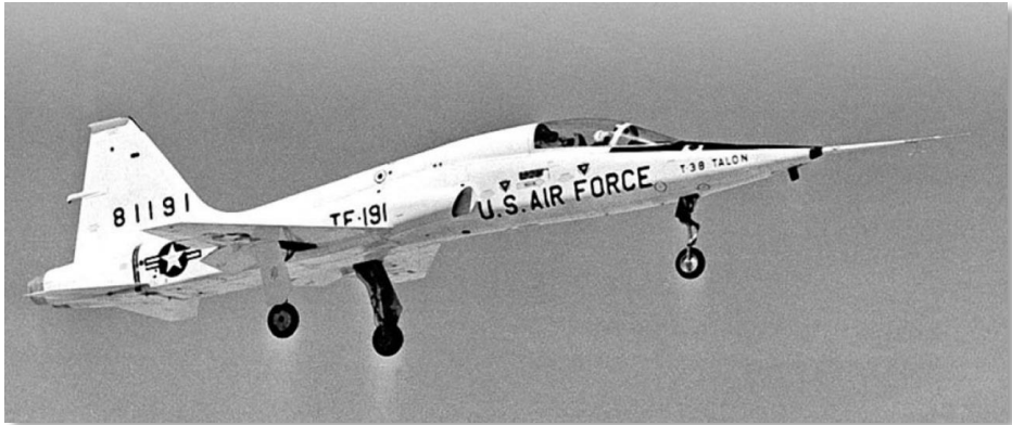
Figure 1.5 The first three YF-38s often flew with closed rear compartment in which different equipment resided
