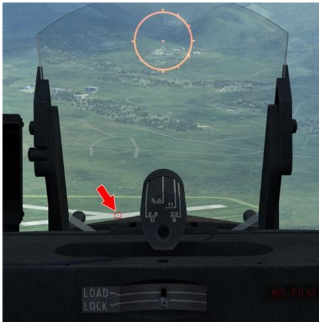
Figure 10.5 Position of the target at the moment when the bombs must be released.
