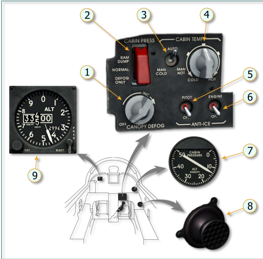
Figure 6.15 Environmental Control System Controls and Indicators in Cockpit
