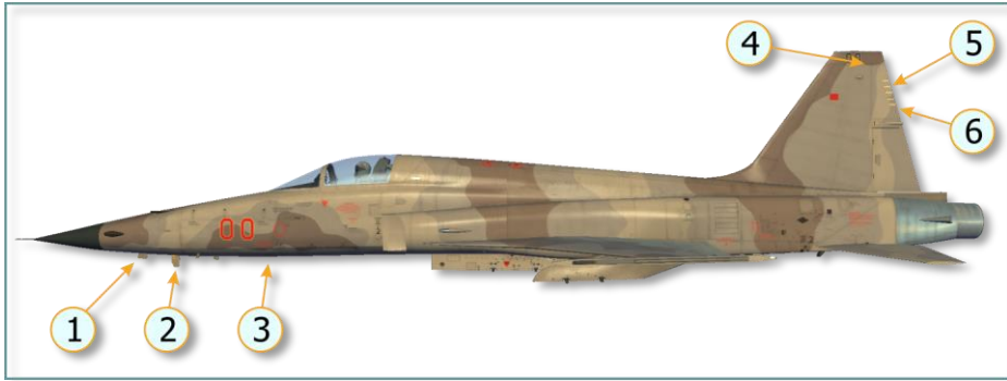
Figure 6.17 Aircraft Antennas Arrangement
