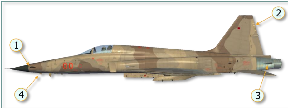
Figure 7.14 AN/ALR-87 Antennas Arrangement
