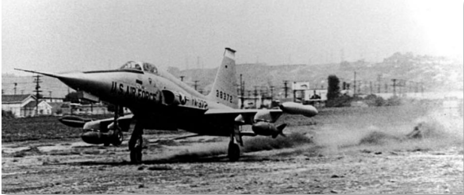
Figure 1.12 Northrop YF-5A (S/N 63-8372) landing on unprepared field. (U.S. Air Force photo) with two 500 lbs bombs and fuel tanks on wingtips
