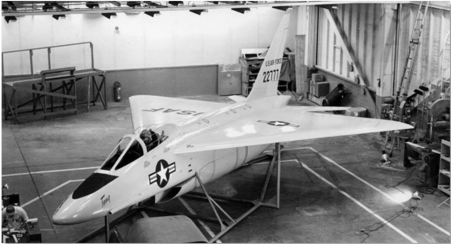
Figure 1.2 N-102 Fang Light fighter mockup – considered to be the F-5 predecessor
