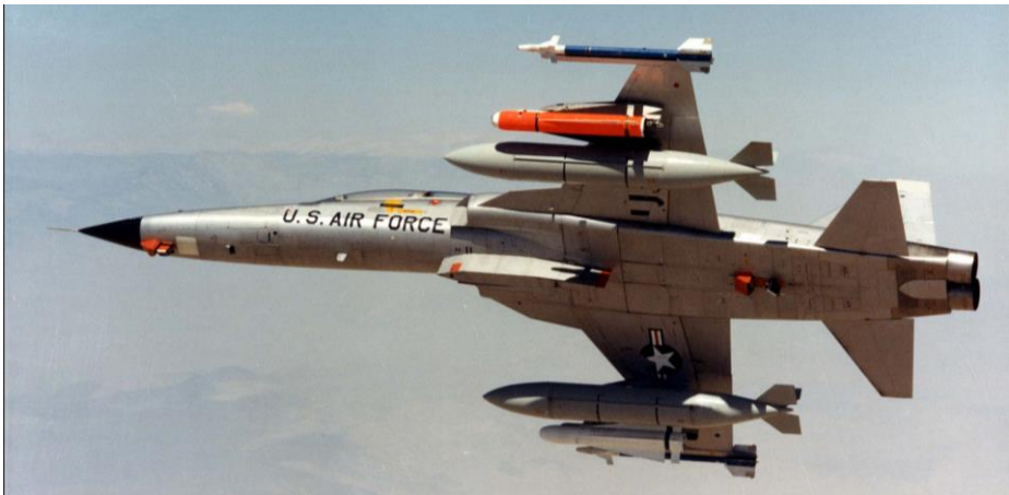
Figure 1.27 F-5F with external tanks, Maverick and Sidewinder missiles. The red box under the nose is a camera for armament usage recording
