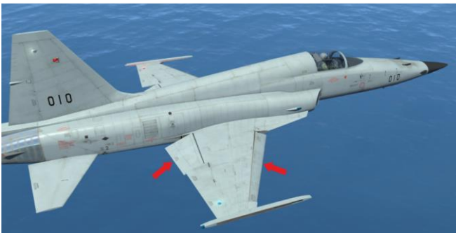
Flaps fully extended – FULL position
