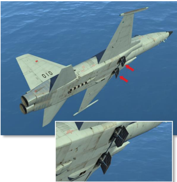
Speed brake open (OUT)
